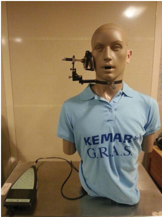
Fig. 2. Setup of the device output level measurement.
